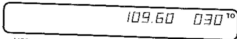
VOR MODE: ACTIVE "BEARING TO" FUNCTION DISPLAY
